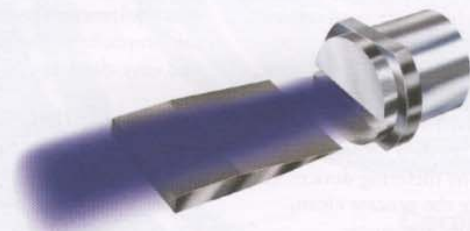
Figure 1: The Sonolator is an in-line homogenising device that employs high pressures and ultrasonic cavitation energy to create emulsions and dispersions.
