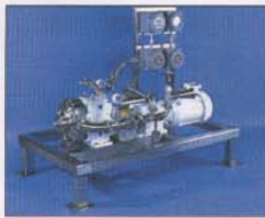
Figure 2: Fumed silica dispersions; Resin manufacturers need a better way to disperse fumed silica into their resin systems as a thickening and anti-sag agent. The Sonolator provided better dispersion, smaller particles sizes and tighter particle size distribution at less than 500psi.
