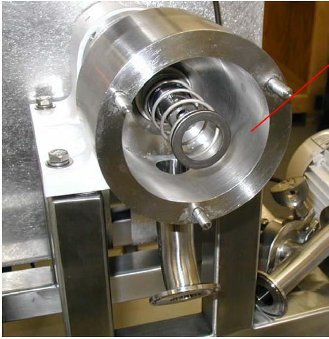
Seal Spring and Spring Retainer
