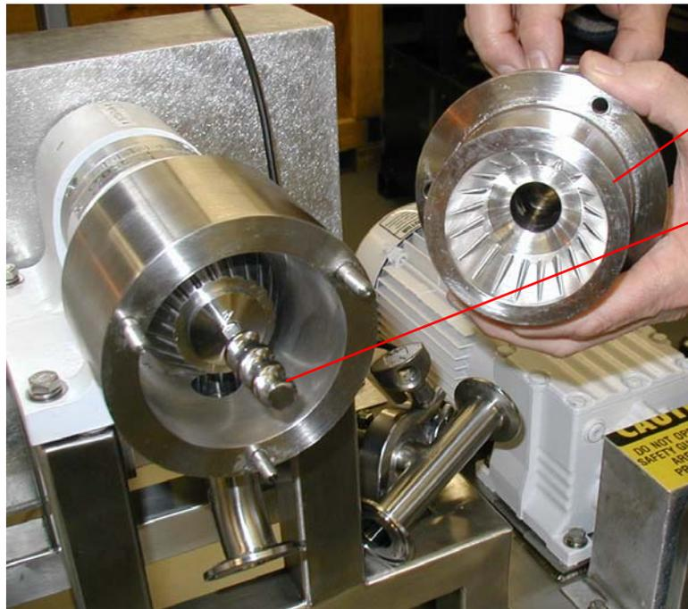
Stator w/ serrated surface
