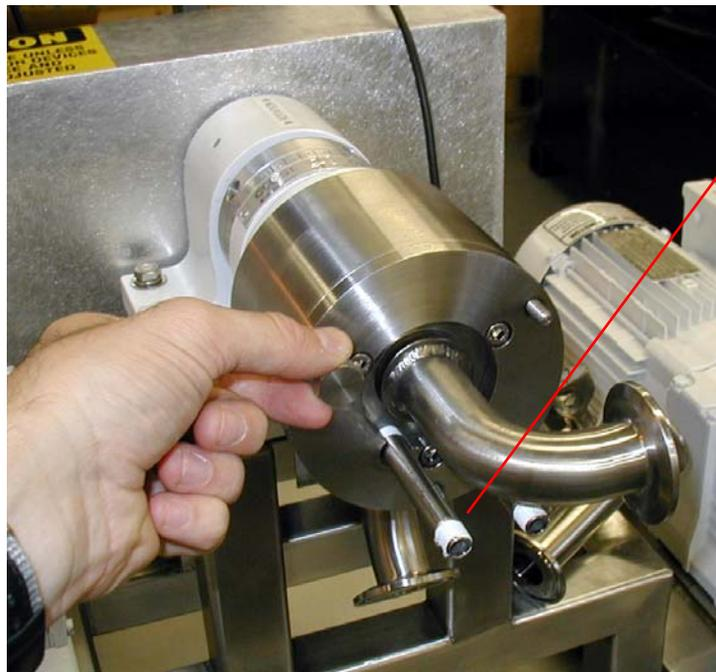
Connect stator cooling water; ¼" NPT
